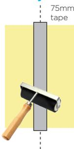
3. Position the 75mm 40 Below™ tape so that the seam between the **Rigid Air Barrier** is at the center of the tape line. The 40 Below™ Tape needs to completely cover the joint.
