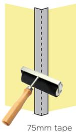
3. Cut the 75mm 40 Below™ Tape to length (add 50mm either side for movement).
