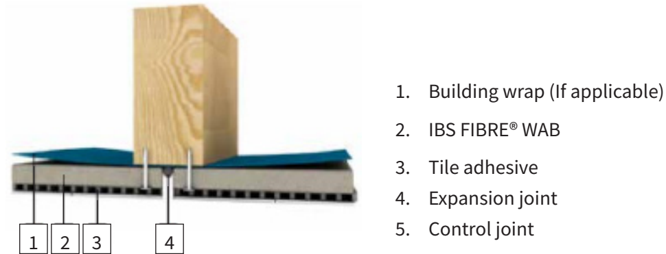
Figure 21 Relief joint details
